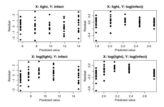
(a) 3 pts. Above are residual vs predicted value plots for four regression models, one for each combination of X = light or  $X = \log(\text{light})$  and Y = infect or  $Y = \log(\text{infect})$ . The combination is described in the title above each plot. What are the X and Y variables in the most reasonable model? Briefly explain your choice.
